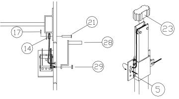
pulleys on vertical lift members, and down to the top 13/32" hole in the pocket and back through the bottom 13/32" hole. Fasten with 3/16" cable clamp (**REF. # 5**). Work winches until cables are raising dock. You must alternate winches as the dock moves up or down. Place VLM pulley cover (**REF. #23**) onto vertical lift member.
