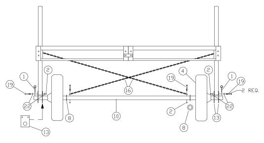
the ends of the axle. Roll axle under dock, keeping axle centered with dock. Bolt lift member bracket (**REF.** # 13) to vertical lift members (**REF.** # 7) with 3/8" X 3" bolts, washers, and nuts (**REF.** # 19, 22, & 2).
