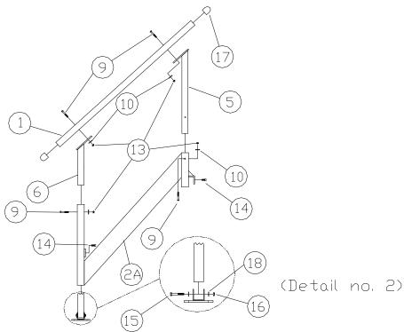
**Step 4.** Place the hook bracket that is on the top of the dock steps over the bottom tube of the dock. Secure in place with 1/2" X 1" set screws. Adjust the bottom leveling leg tube until your dock steps are approximately level. Tighten setscrews at this time.
