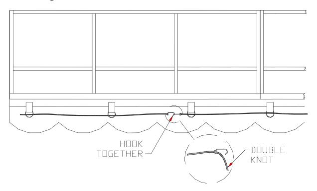
Using "S" hooks, fasten the shock cord to the frame between <u>each</u> of the "D" rings on the canopy. Hook a few on each end, then a few on each side, alternating back and forth to evenly tension the canopy. Be sure to use one "S" hook between every two "D" rings.
