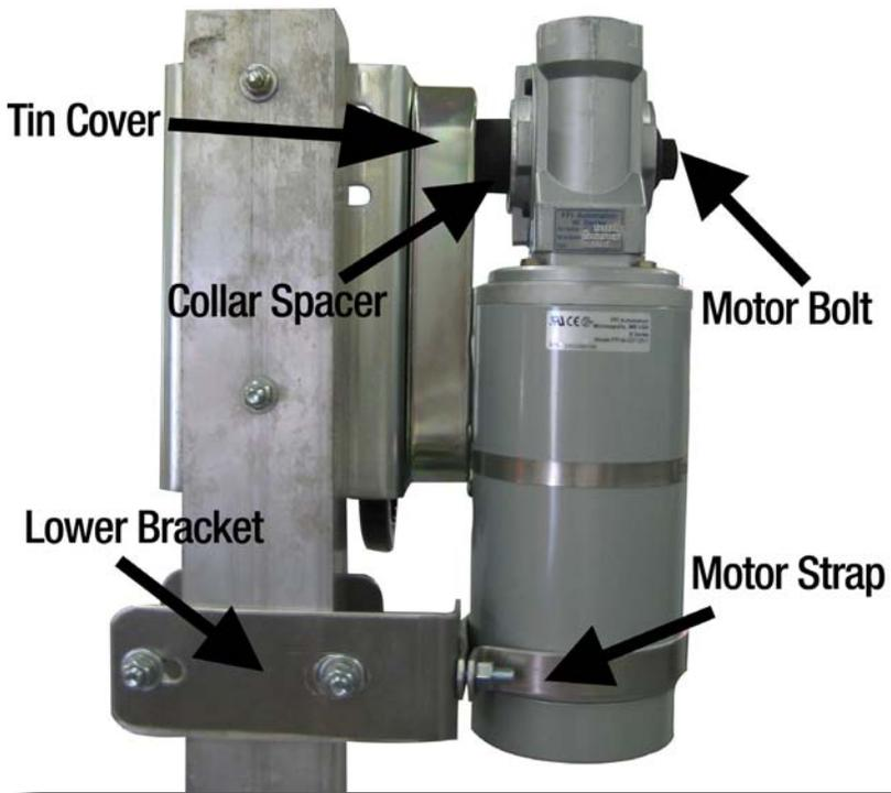
9. Slide Motor onto the Spline.
