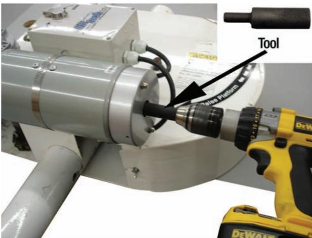
In case of a Power Outage, this Tool may be Inserted into a Drill to Raise or Lower your Lift.
