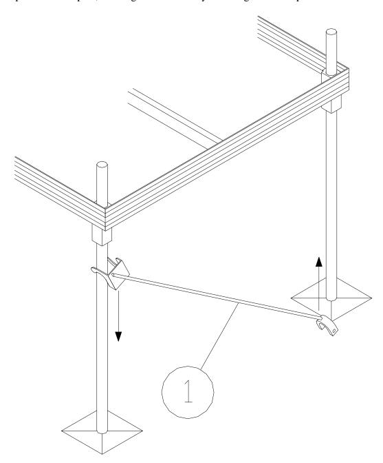
Step 2. Once both stabilizer bars are on the legs secure in place with 1" set screws.
