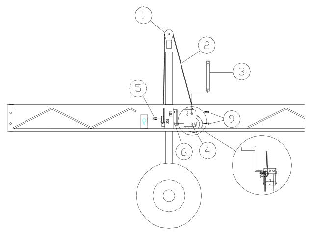
**STEP 2.** Bolt chains (**REF.** # 7) to the inside holes on the axle using a 3/8" x 3" bolt and nut. Run the other end of the chain up to the opposite side of the dock through the keyhole bracket located next to the vertical lift member pocket.
